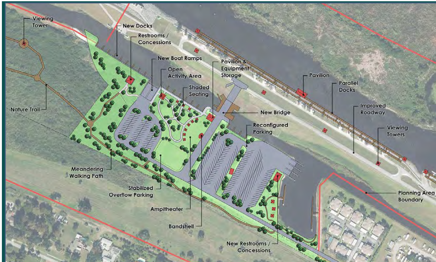
Concept #1 had the least amount of inland impact and was a consideration for minimizing permitting requirements.
